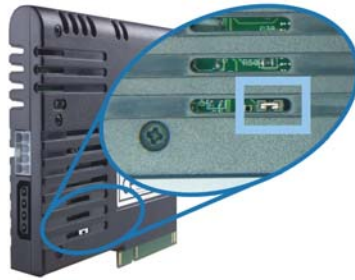
Figure 7. Location of the removable circuit jumper on PCI card
